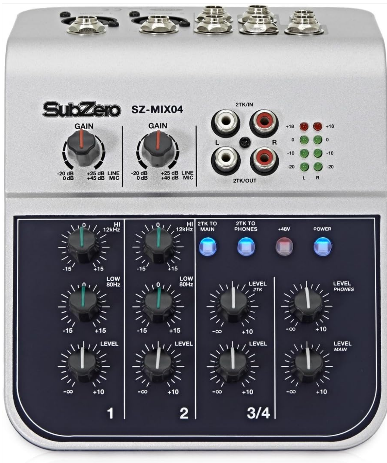
Figure 3.2: Top view of the SZ-MIX04, highlighting the gain, EQ, and level controls for each channel, along with the main output and headphone controls.
