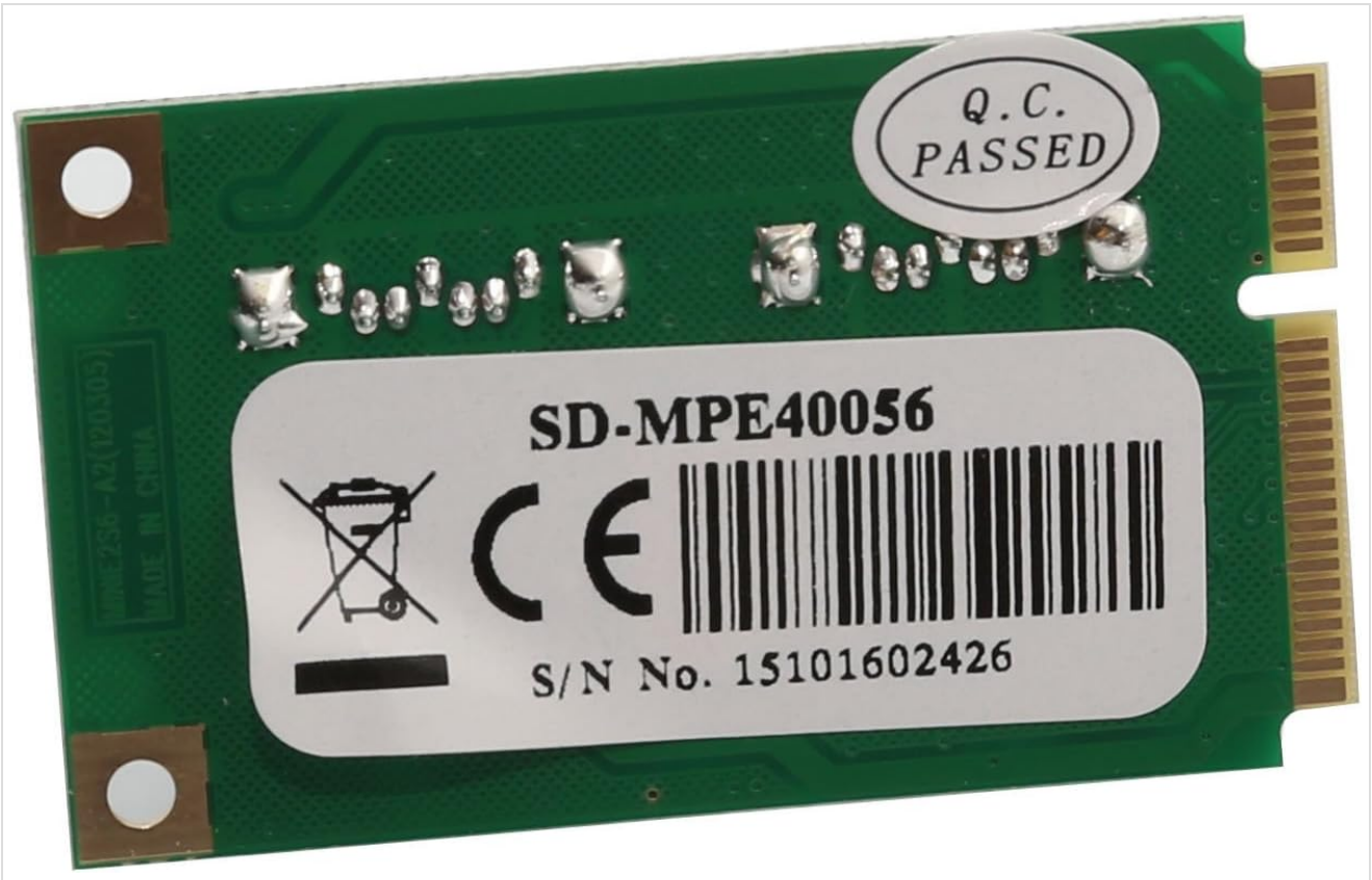
Image: Rear view of the Syba Mini PCIe SATA III Controller Card, showing the model number SD-MPE40056 and serial number 15101602426 on a label.
