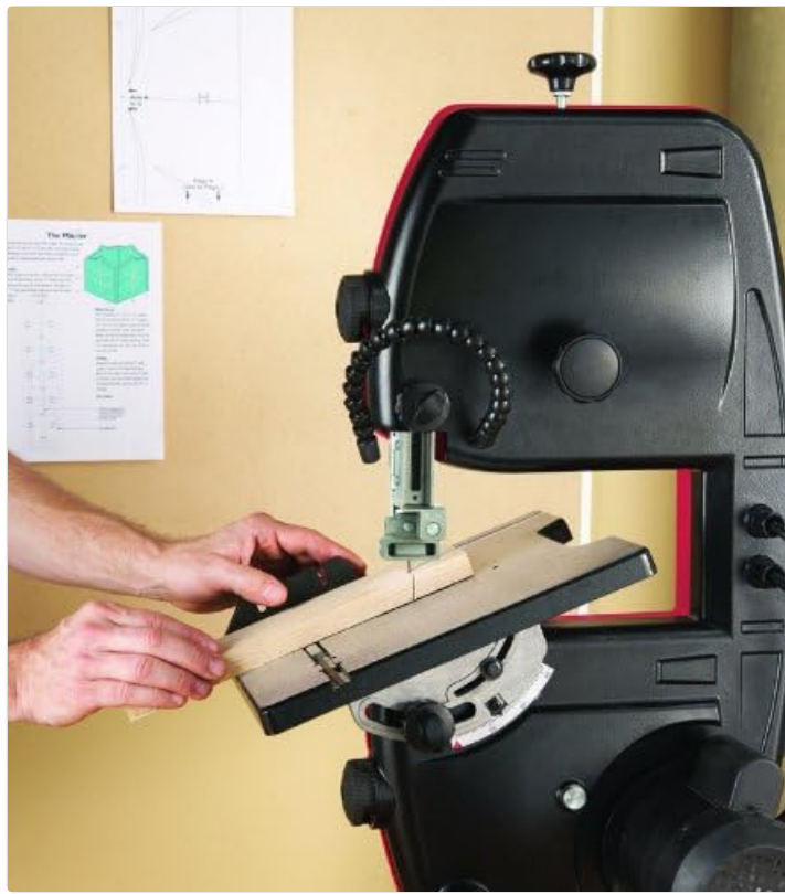
Figure 4: Adjusting the table for angled cuts using the miter gauge, allowing for versatile woodworking applications.
