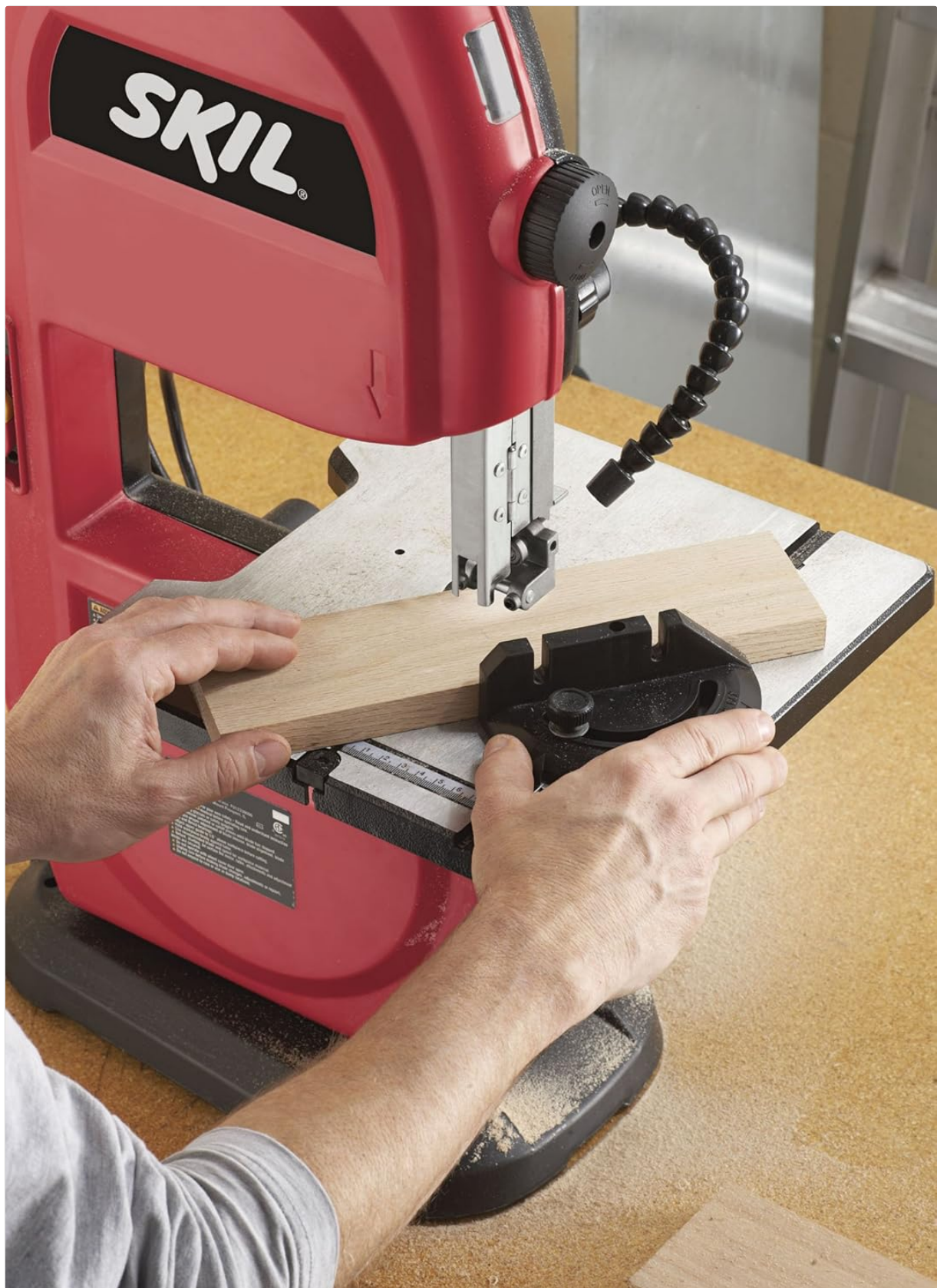
Figure 1: Overview of the SKIL 3386-01 9-Inch Band Saw during operation, demonstrating proper hand placement for guiding material.
