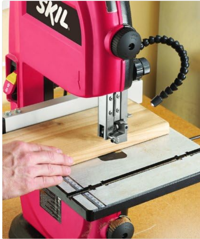
Figure 3: Utilizing the rip fence for precise straight cuts, ensuring consistent material width.
