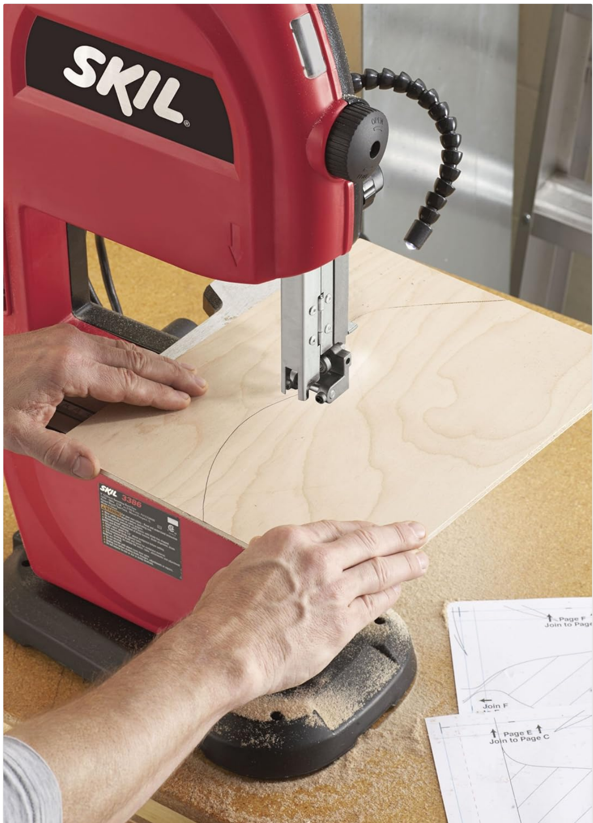
Figure 2: The band saw in action, illustrating its capability to cut intricate and curved patterns in wood.
