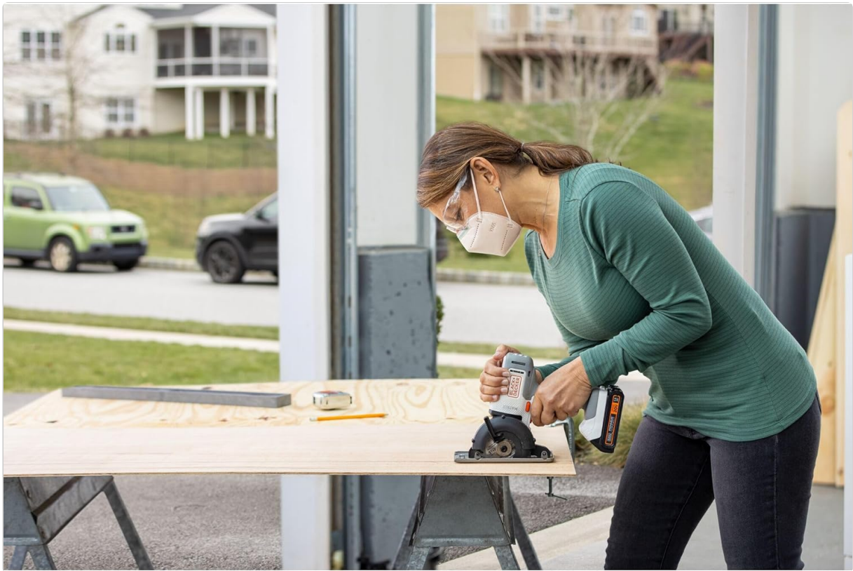
Figure 5: Proper technique for using the trim saw attachment to cut a wooden board.
