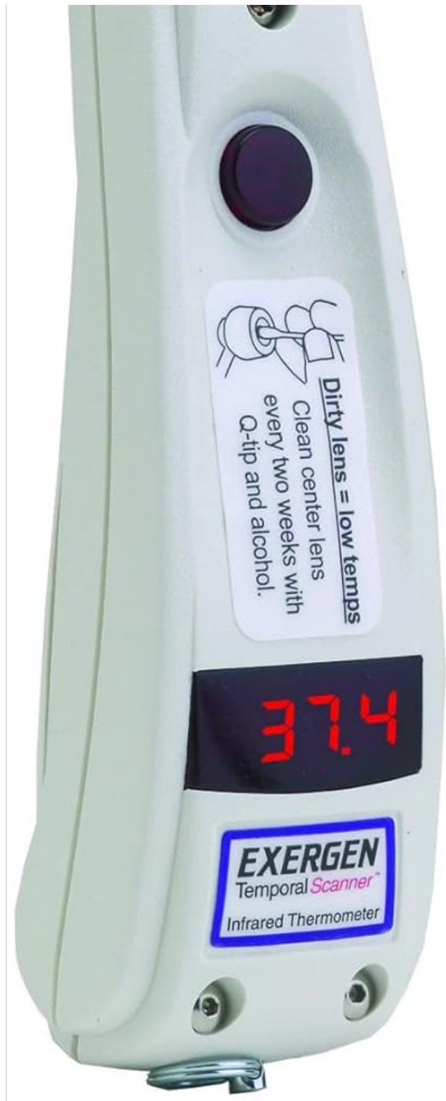
Figure 1: Exergen TemporalScanner Infrared Thermometer. The image displays the device with its sensor head, main body, and digital display showing "37.4". A label on the device indicates "Dirty lens = low temps" and provides instructions to "Clean center lens every two weeks with Q-tip and alcohol."
