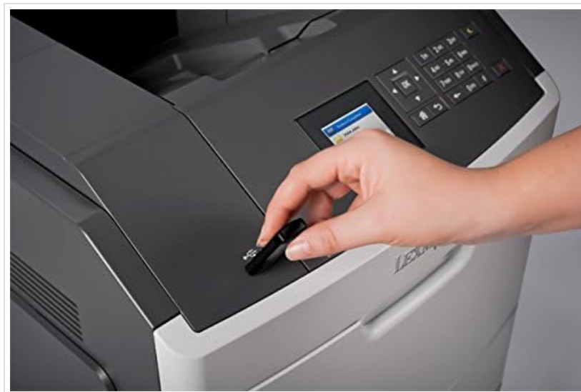
Figure 3: A hand inserting a USB flash drive into the dedicated USB port located on the top surface of the printer, near the control panel.
