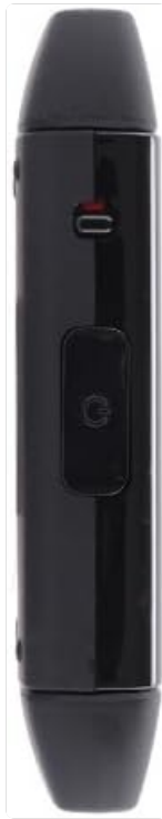
Figure 3.3: Side view of the device, indicating the location of the power button.
