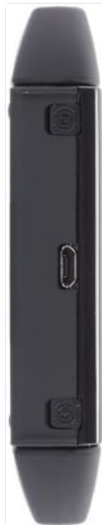
Figure 3.2: Side view of the device, highlighting the micro-USB charging port.
