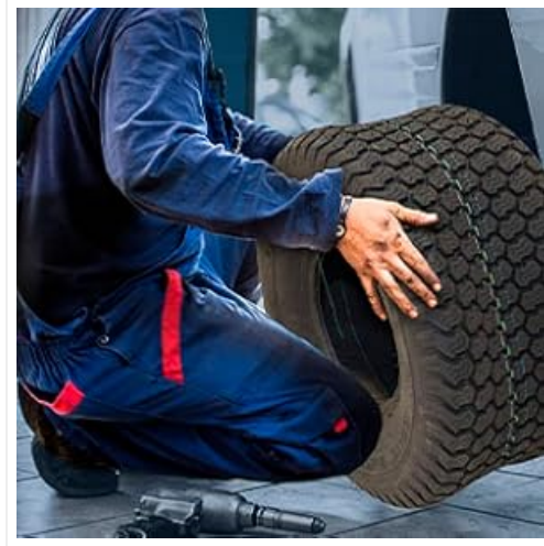
Image 2: A technician carefully installing a tire onto a rim, demonstrating proper handling during the mounting process.
