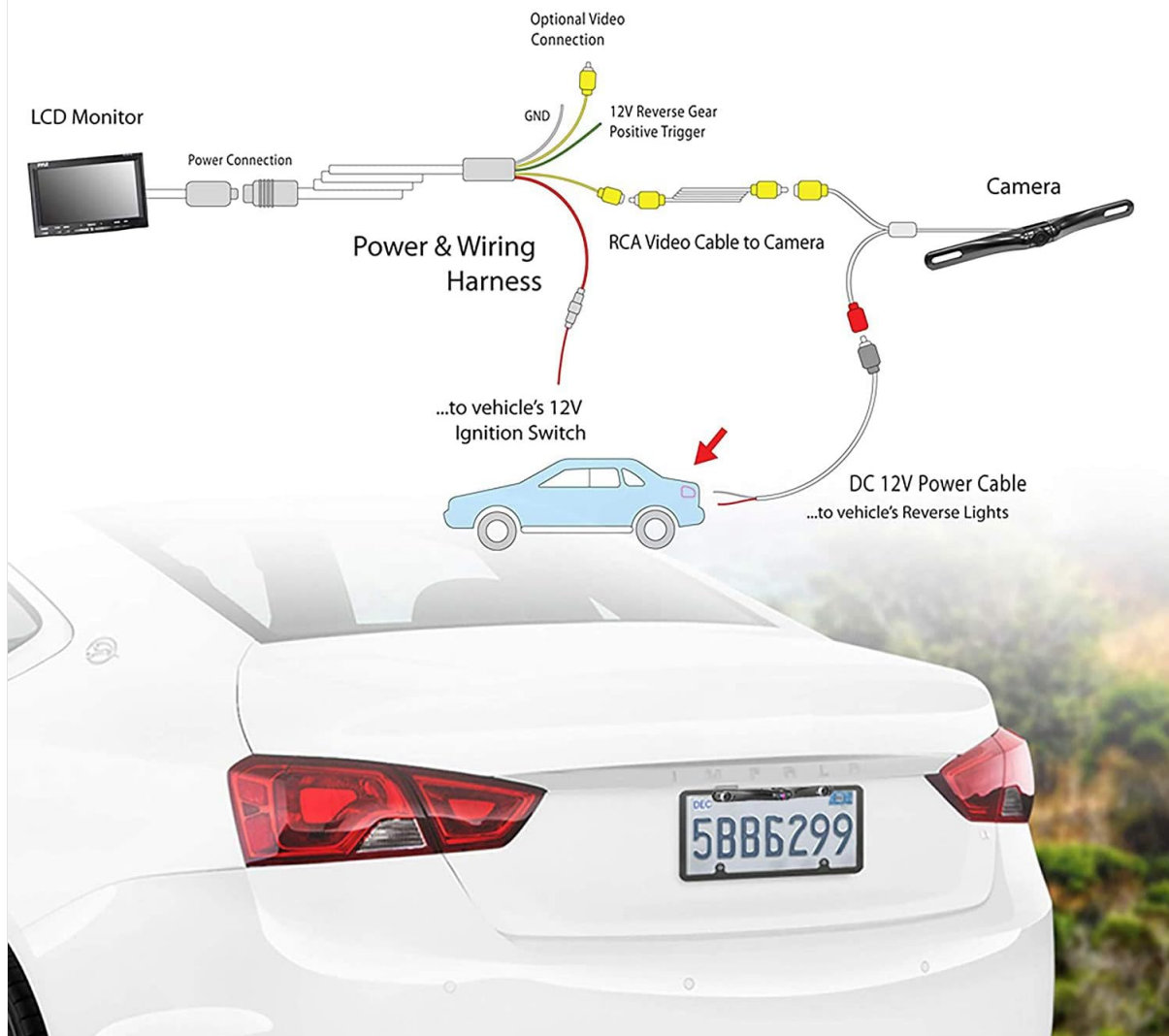
Figure 5: Wiring connections for the Pyle PLCM7500 system.
