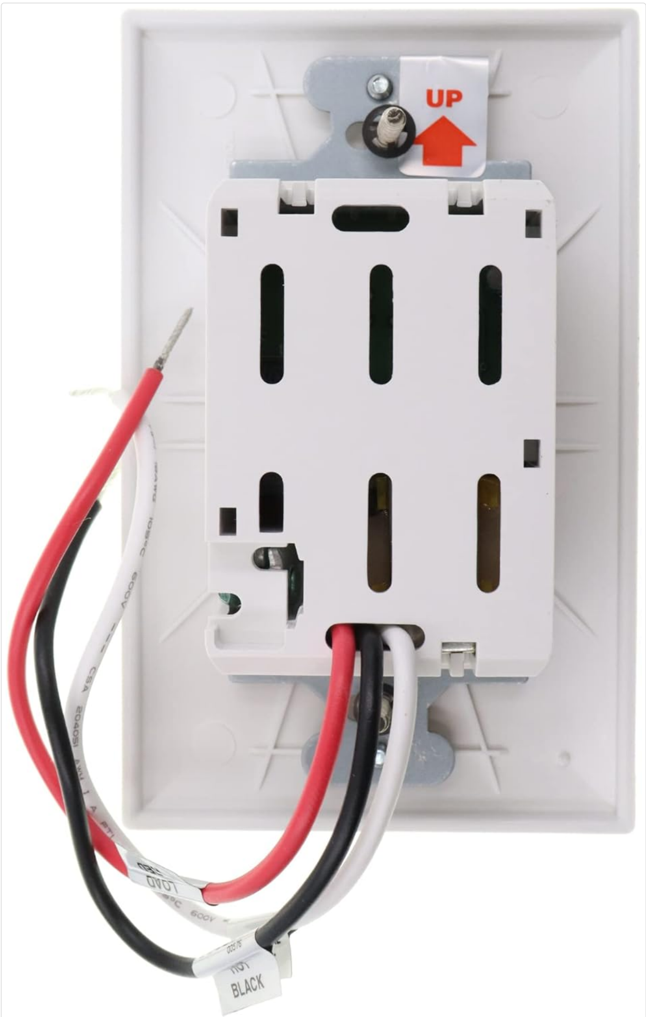
Figure 1: Back view of the sensor illustrating the wiring connections (Black for Line, Red for Load, White for Neutral, Green for Ground).
