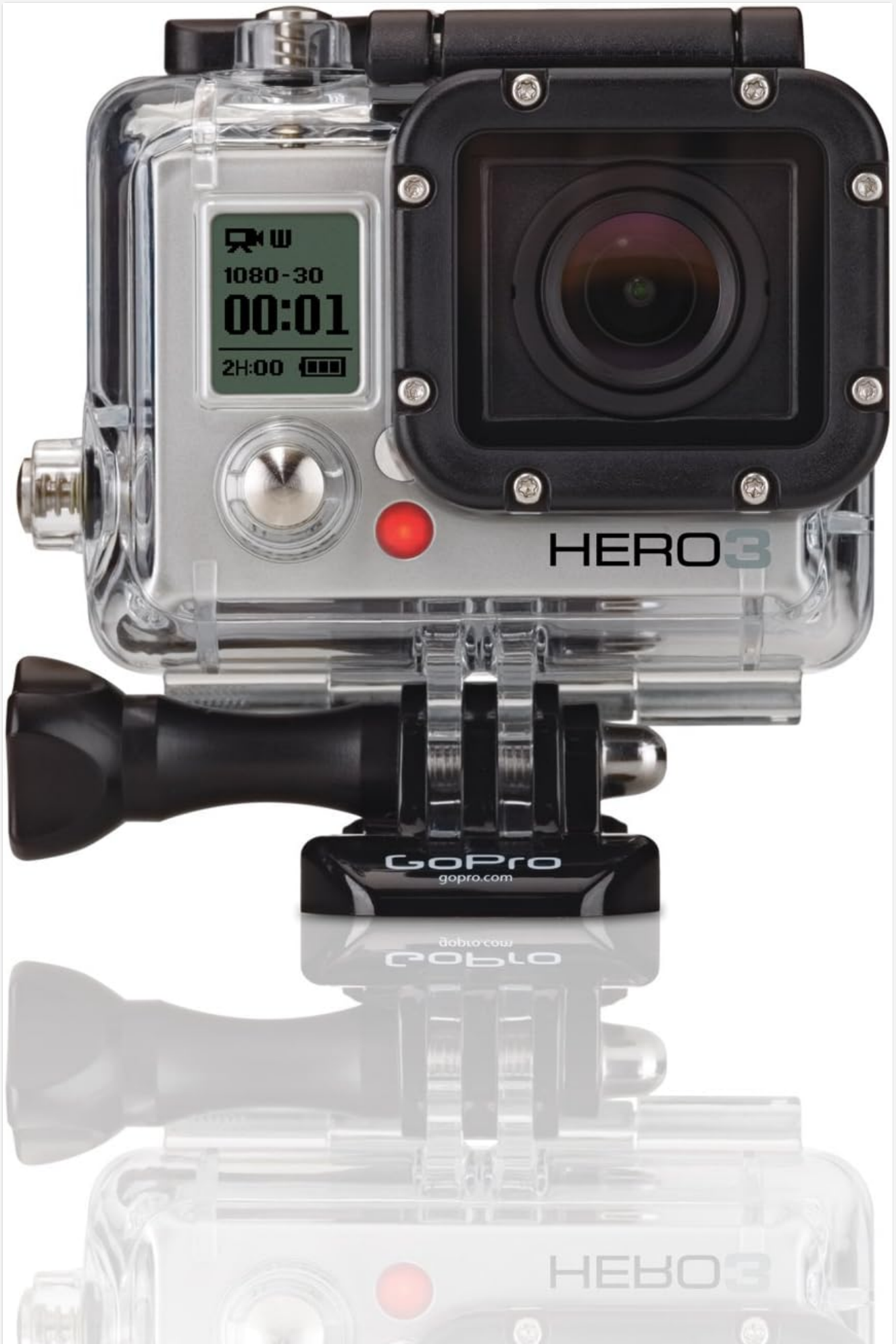
Figure 3.1: Front-angled view of the GoPro HERO3 Silver Edition in its waterproof housing.
