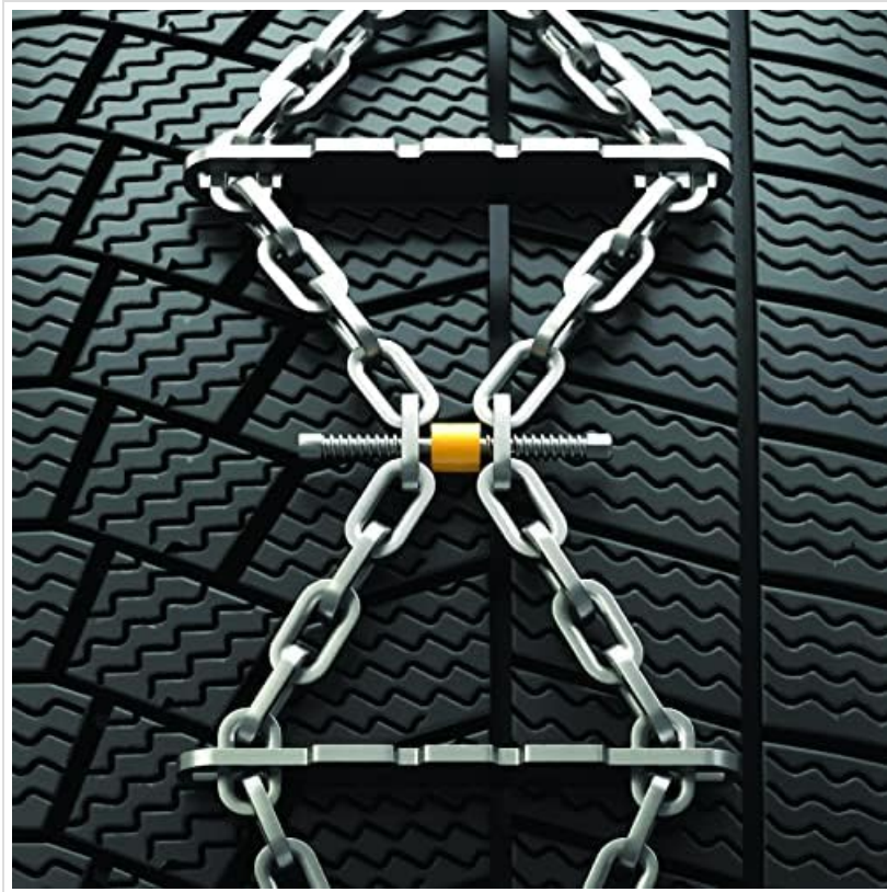
Figure 3: Close-up view of the KÖNIG K-Summit K11 chain links and injection-moulded plastic plates.
