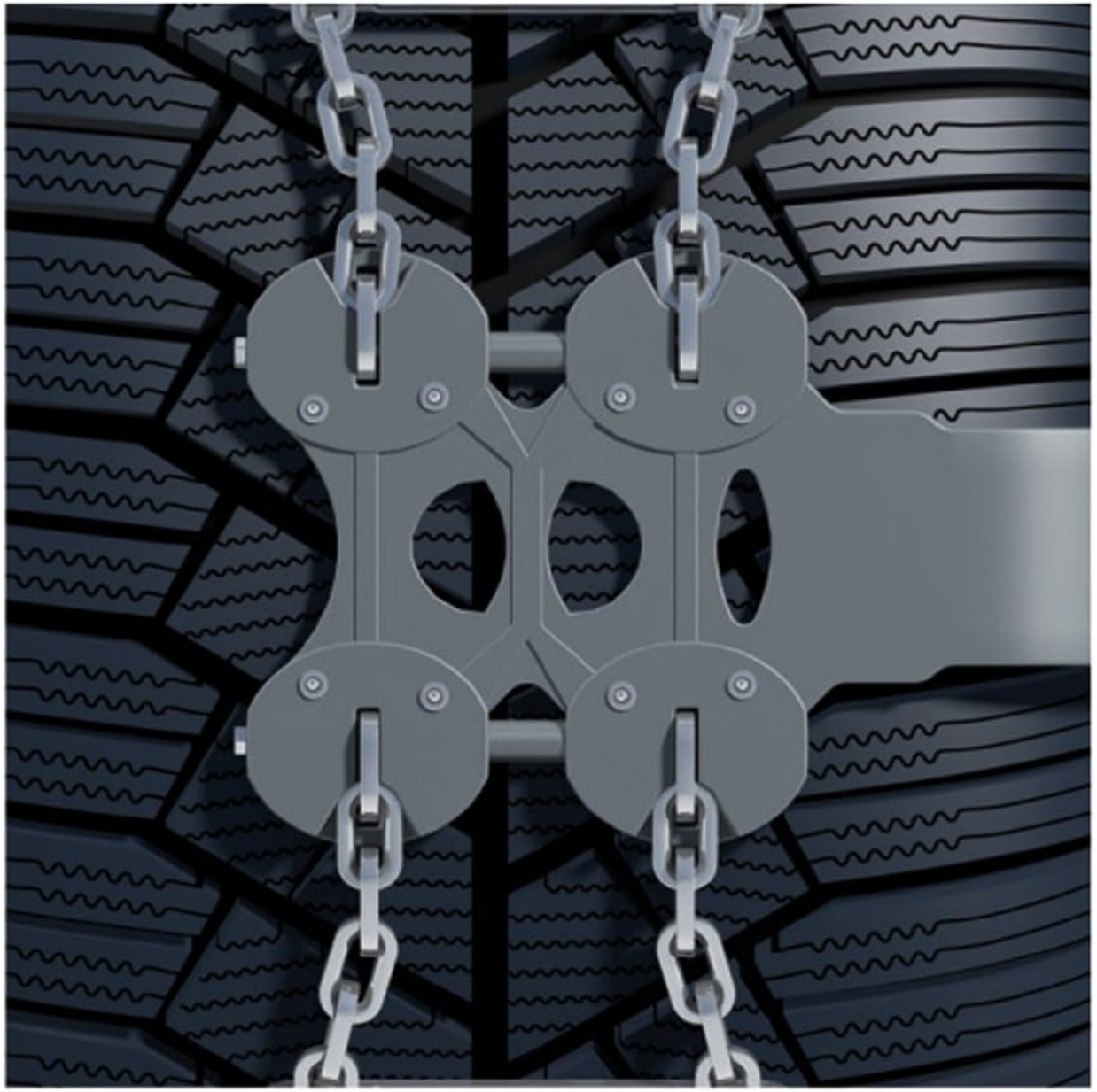
Figure 4: Detail of the chain links and plastic plates on the tire tread during installation.
