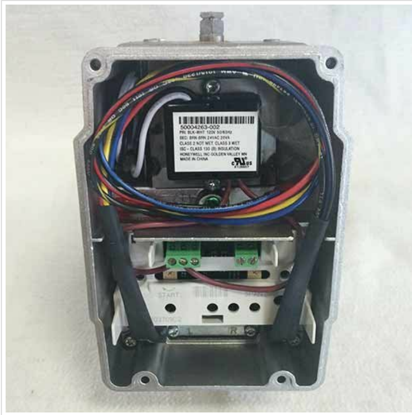
Figure 4: View of the motor's internal wiring and terminal connections.
