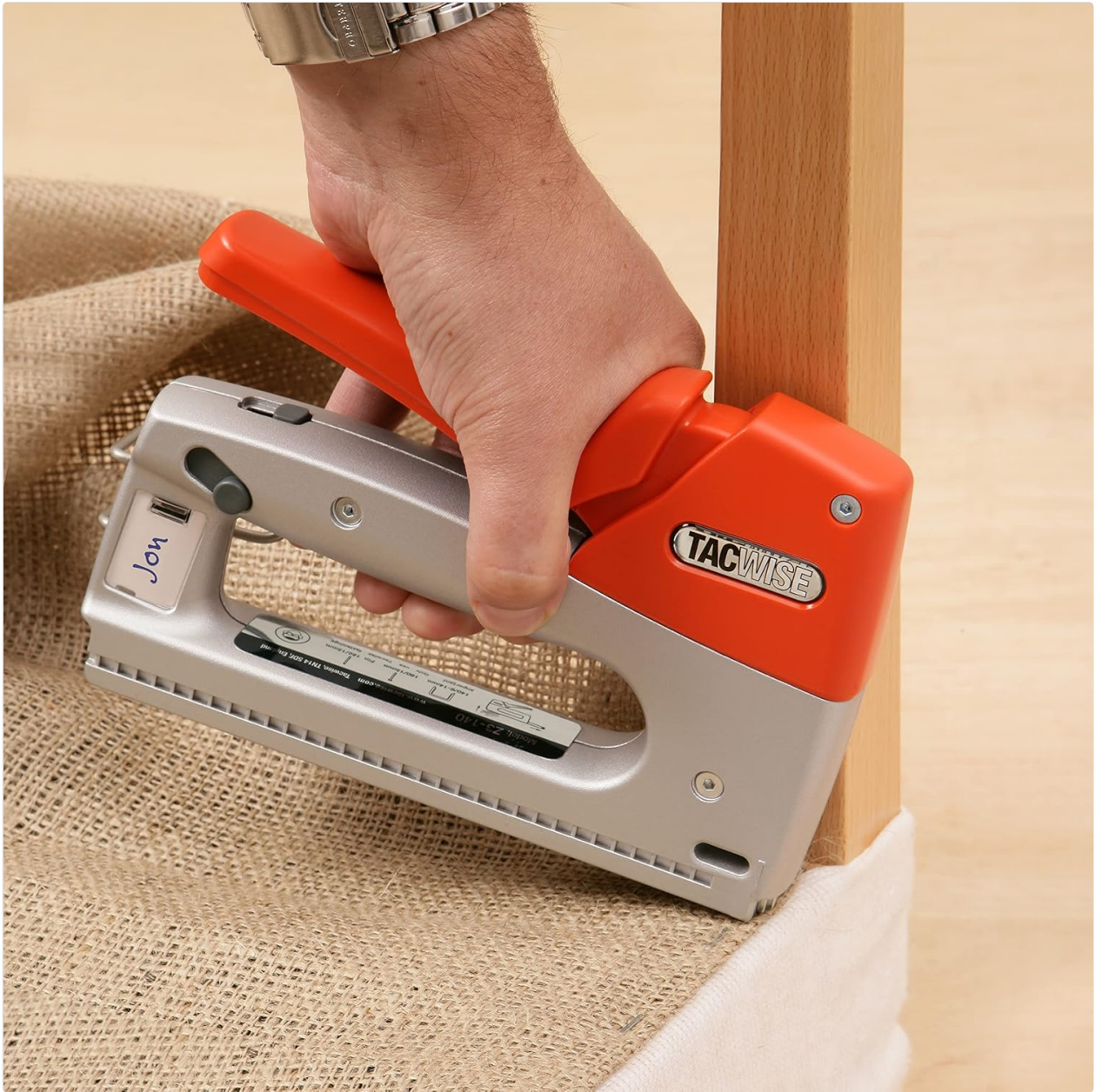
Figure 6: Tacker being used for upholstery application.
