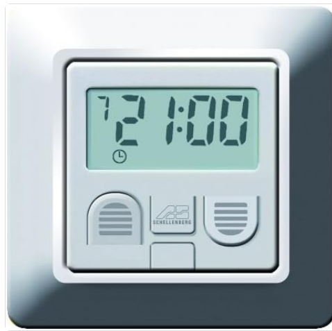
Image: A close-up front view of the Schellenberg Zeitschaltuhr Plus, showing its digital display and three control buttons.
