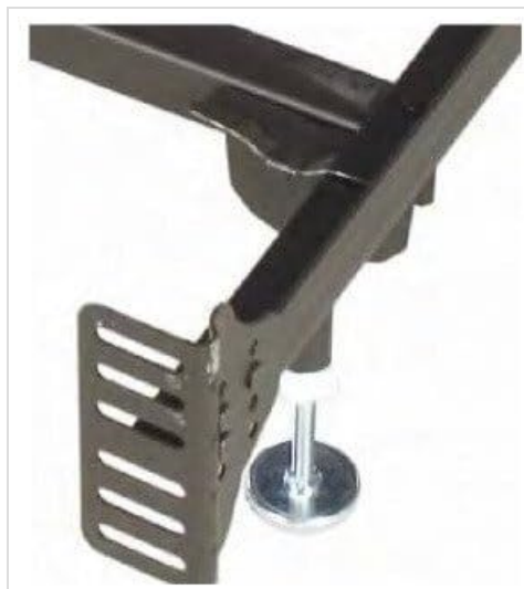
Figure 2: A detailed view of the multi-slotted bracket and an adjustable glide on a leg of the Glideaway BB24 bed frame. This shows how the frame connects to a headboard or footboard and how the height can be adjusted for stability.
