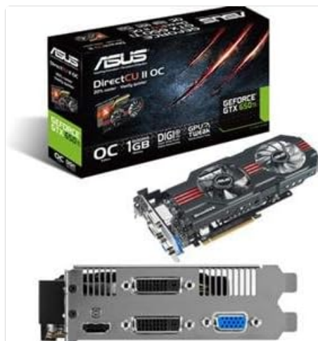
Image: The ASUS NVIDIA GeForce GTX 650 Ti OC graphics card, its retail packaging, and a detailed view of its VGA, DVI, and HDMI output ports.
