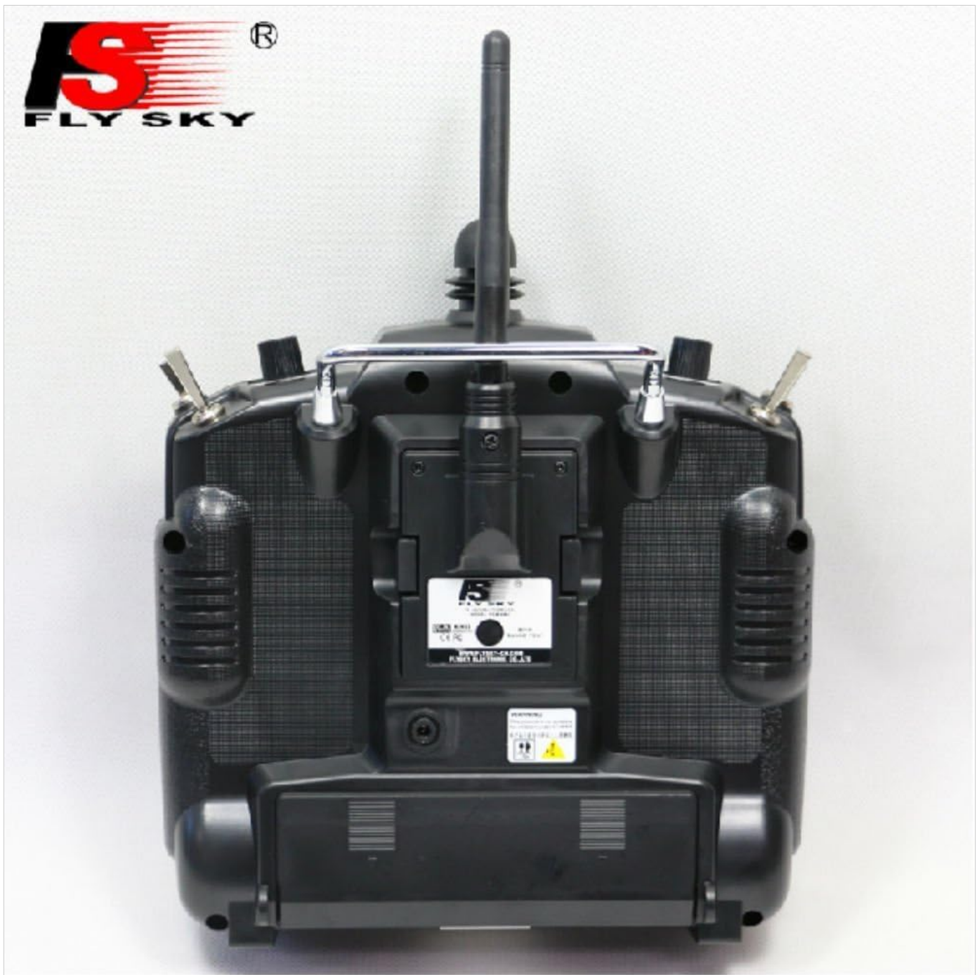
Figure 3.1: Rear view of the FS-TH9X transmitter, highlighting the battery compartment and other ports.
