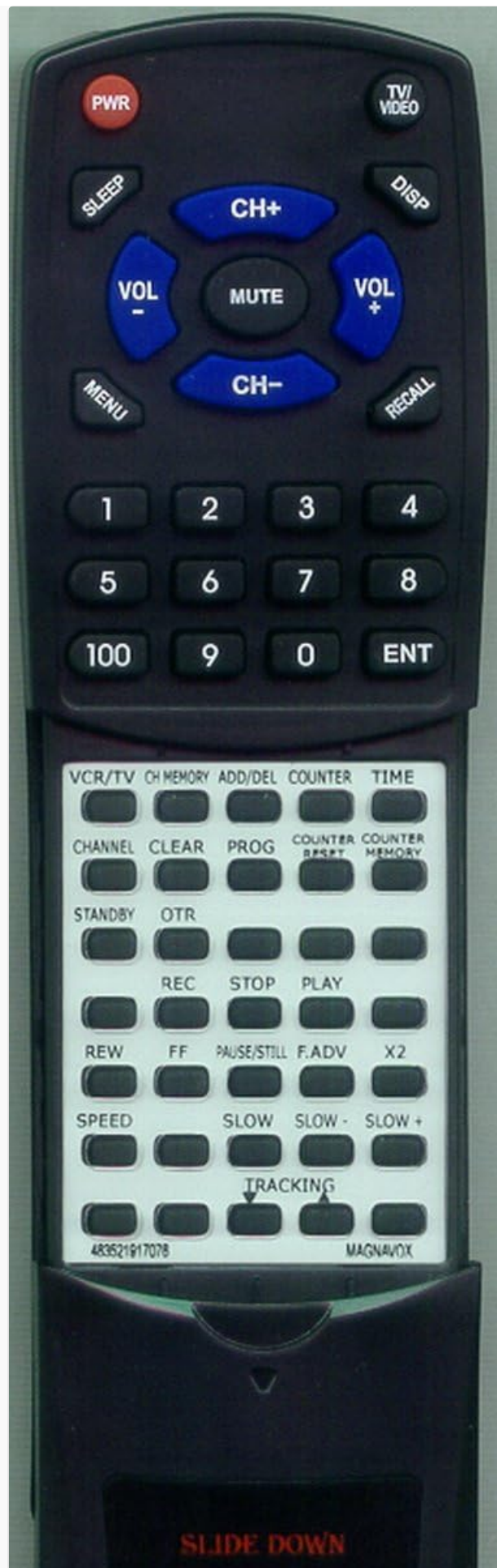
Image: Front view of the Redi-Remote replacement remote control. The remote is dark gray with black and blue buttons. The top section features power, channel, volume, mute, menu, display, and recall buttons, along with a numeric keypad. The lower section, initially covered by a sliding panel, reveals additional VCR function buttons such as play, record, fast forward, rewind, pause, and tracking controls.
