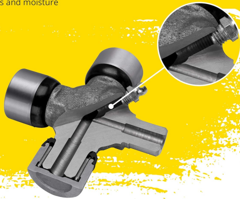
Image: A cutaway diagram of the universal joint, illustrating the internal grease channels and fitting for easy lubrication.
