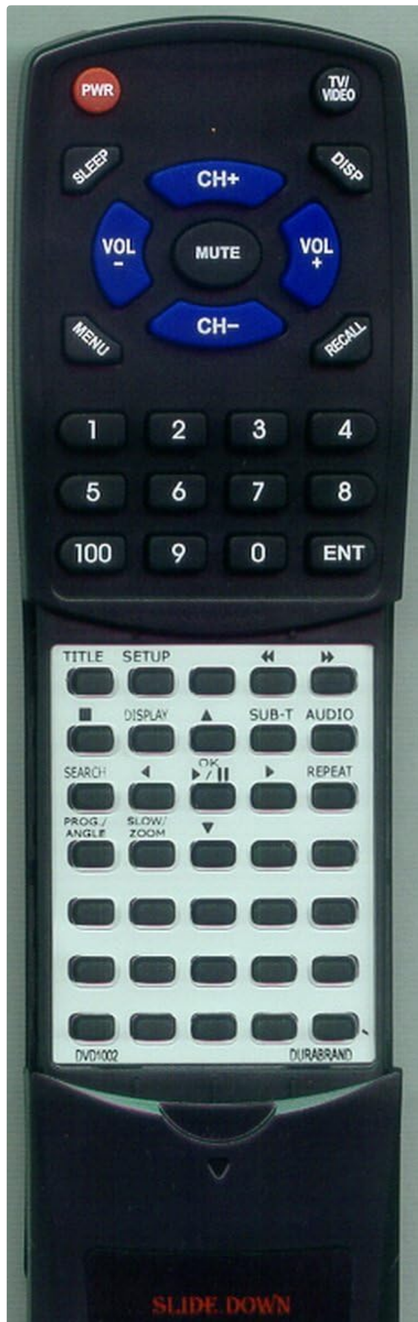
Figure 1: Redi-Remote Replacement Remote Control. This image displays the full remote control, featuring the upper section with primary navigation and number buttons, and the lower section, which slides down to reveal additional playback and setup controls.
