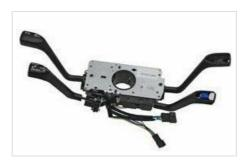
An overhead view of the Porsche 996 Combination Switch, showing its central mounting plate and four control stalks extending outwards, with various electrical connectors visible.
