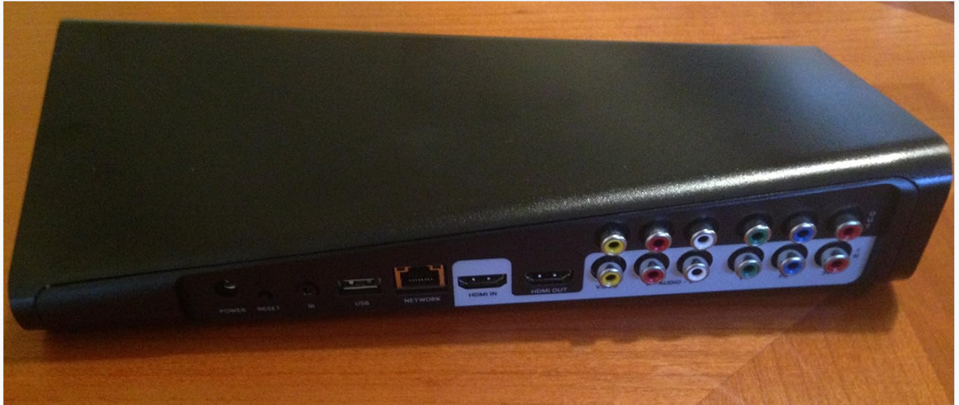
Figure 3.1: Rear panel of the Slingbox 500, showing various input and output ports including Power, Reset, USB, Network (Ethernet), HDMI In, HDMI Out, and Audio/Video (component/composite) connections.
