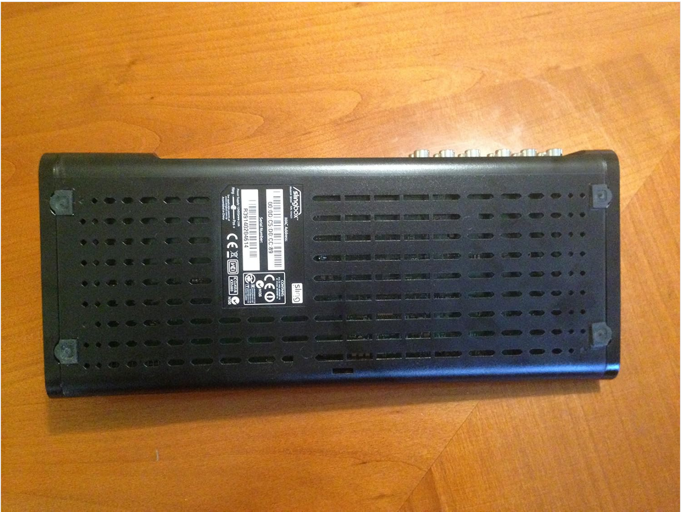
Figure 6.1: Bottom view of the Slingbox 500, showing ventilation grilles for heat dissipation and product labels.
