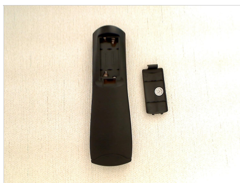
Figure 2: Battery compartment with cover removed.
