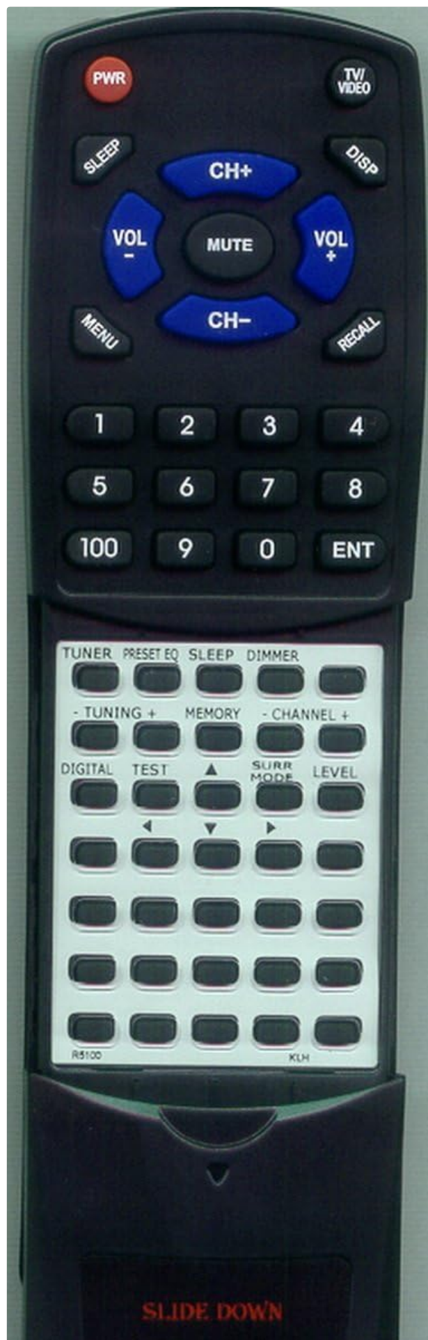
Figure 1: Redi-Remote Replacement Remote Control showing both visible and hidden buttons.
