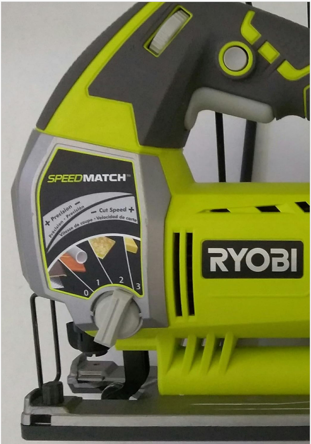
Figure 2: A detailed view of the jigsaw's side, highlighting the 'SpeedMatch' dial. This dial allows users to select between 'Precision' and 'Cut Speed' settings, with numerical indicators (0-3) for orbital action adjustment, optimizing cuts for different materials and desired finishes.
