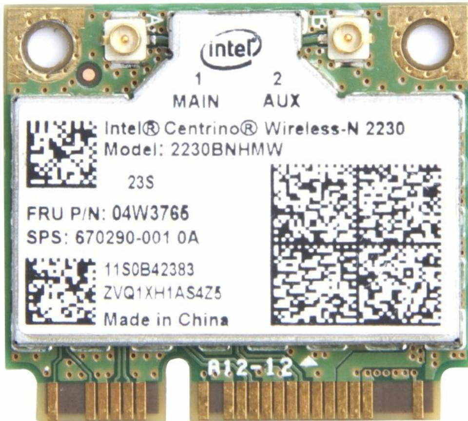
Image: Intel Centrino 2230 Mini PCI Express Wi-Fi/Bluetooth Combo Adapter. The image displays the top side of the card, highlighting the "MAIN" (1) and "AUX" (2) antenna connectors, the Intel logo, and the model number "2230BNHMW" clearly printed on the label.
