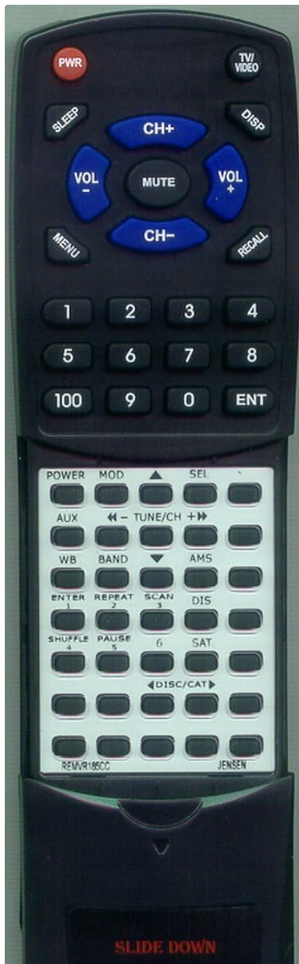
Figure 1: Full view of the Redi-Remote replacement remote control. The top section features primary controls, while the lower section is revealed by sliding down the cover.
