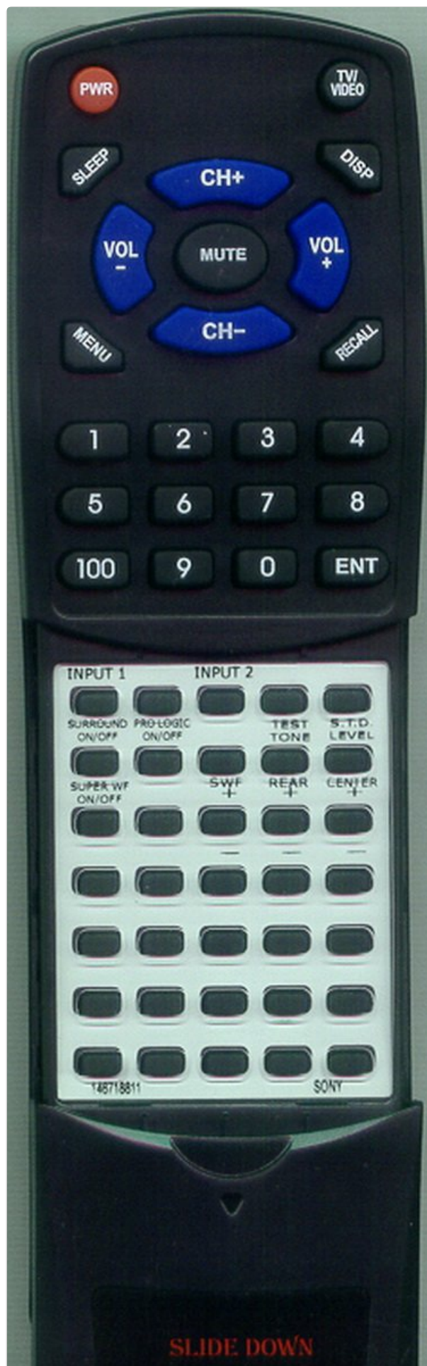
Image 2: The Redi-Remote control with its sliding cover moved down, revealing the secondary set of buttons for advanced functions.
