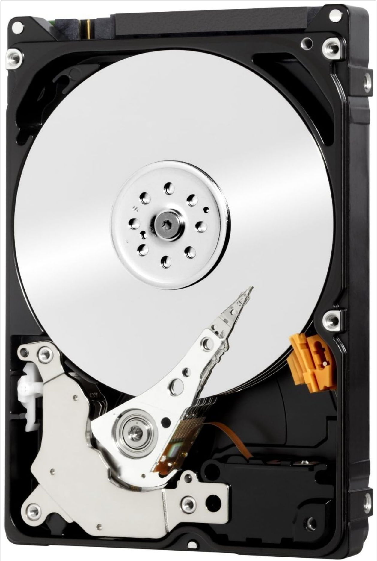
Figure 1: Top-down view of the Toshiba DT01ACA100 hard drive, illustrating internal components.
