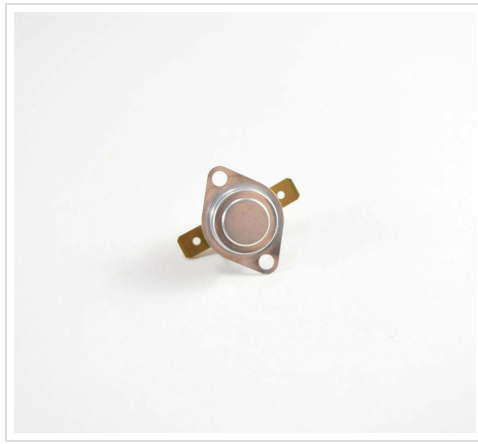
Image: A close-up view of the Goodman B1370145 Furnace Burner Roll-Out Limit Switch. It is a small, circular metal disc with two mounting holes and two electrical terminals, designed to detect overheating.
