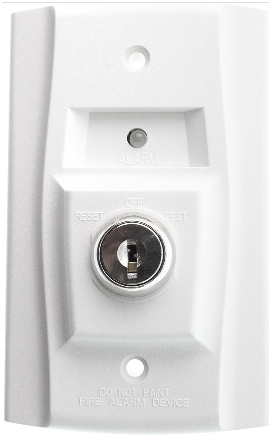
Figure 4.1: Front view of the RTS151KEY Remote Test Station. It features a key switch with OFF, RESET, and TEST positions, and an ALARM indicator LED.
