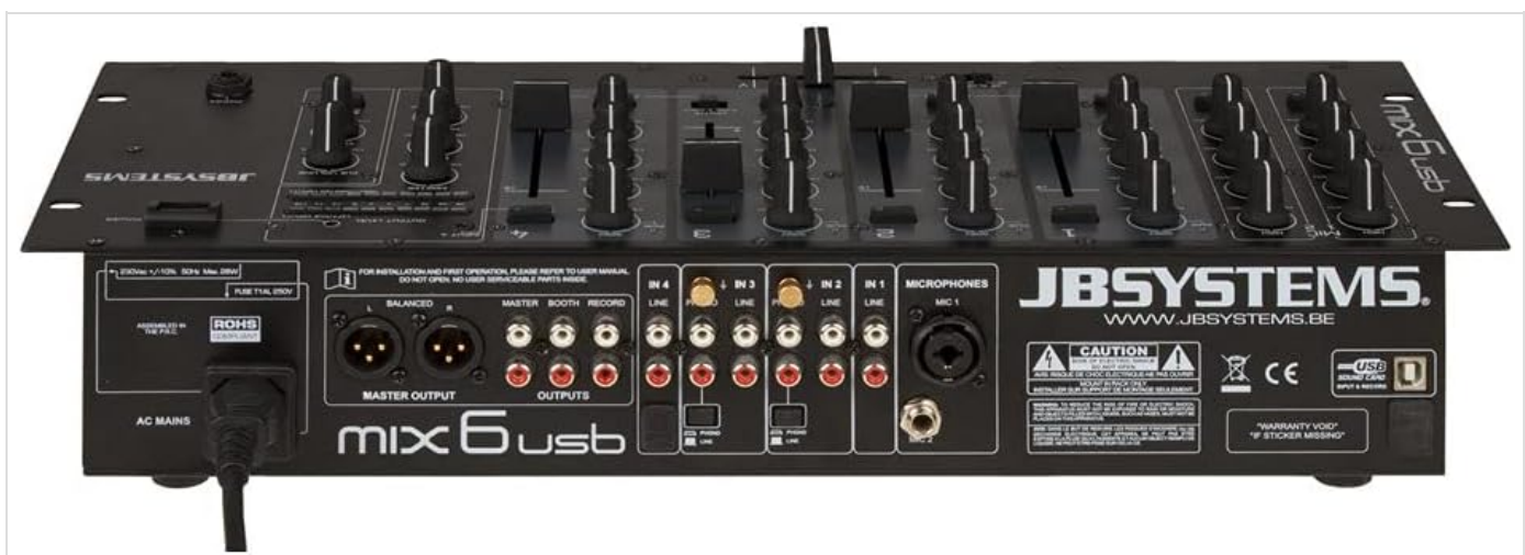
Figure 3.4: Rear panel of the MIX-6 USB mixer, displaying various input and output connections including XLR master outputs, RCA inputs, and USB port.
