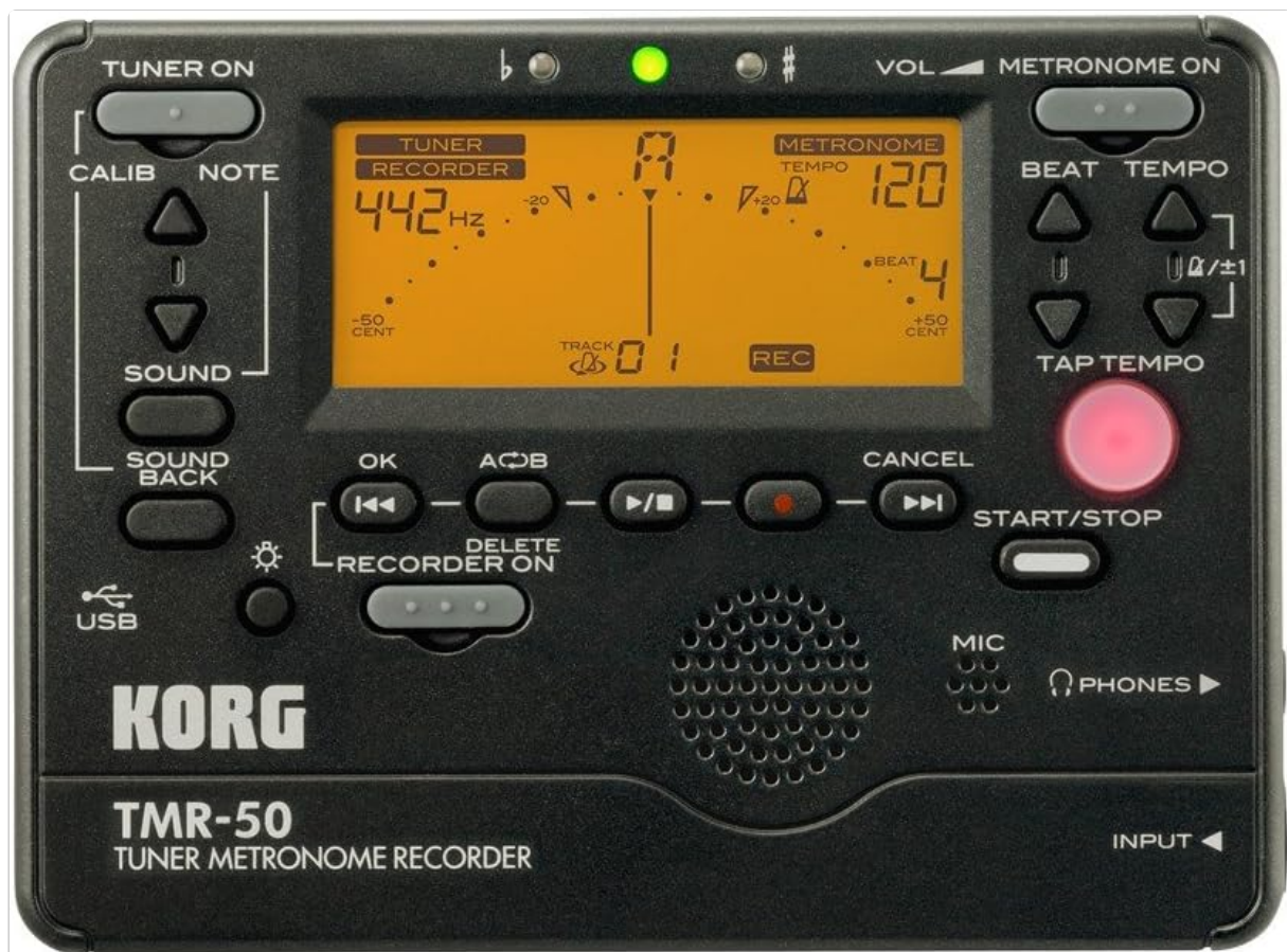
Figure 1: Front panel overview of the Korg TMR-50, showing all controls and the display.
