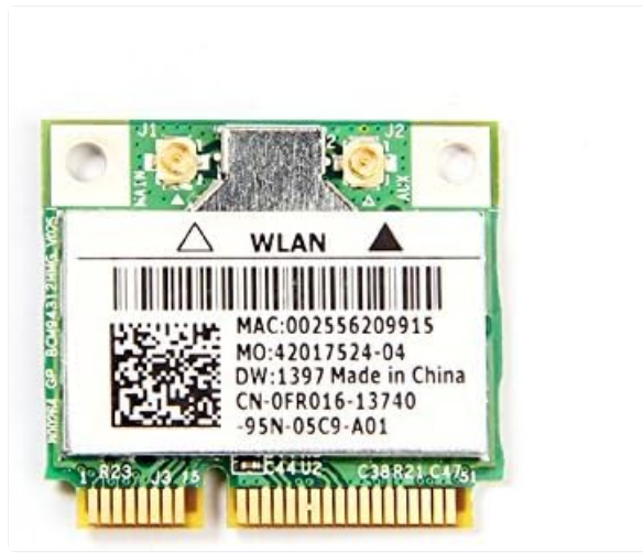
Figure 2: Rear view of the Dell DW1397 Broadcom Wireless Card. This side features a label with important identification details such as the MAC address, model number (DW:1397), and manufacturing information. Two antenna connectors are visible at the top edge of the card.
