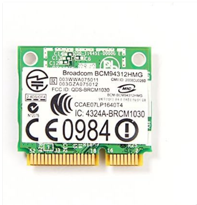
Figure 1: Front view of the Dell DW1397 Broadcom Wireless Card. This image displays the primary components and regulatory markings, including the Broadcom BCM94312HMG chip, FCC ID, and various international certifications. The gold-plated Mini PCI Express contacts are visible at the bottom.
