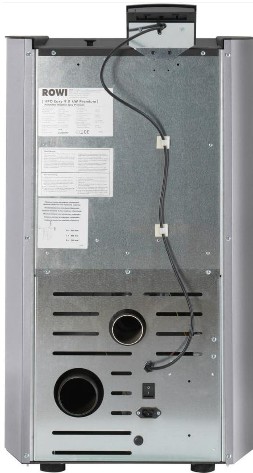
Figure 3.4: The rear view of the pellet stove, illustrating the exhaust pipe connection (80mm diameter), the external air intake, and the power connection point.
