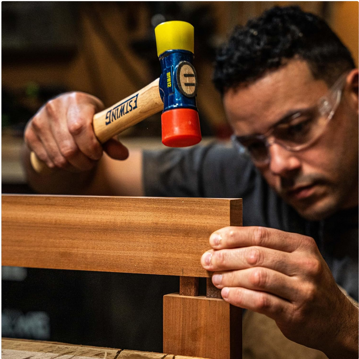
Figure 4: Mallet in use for wood assembly
