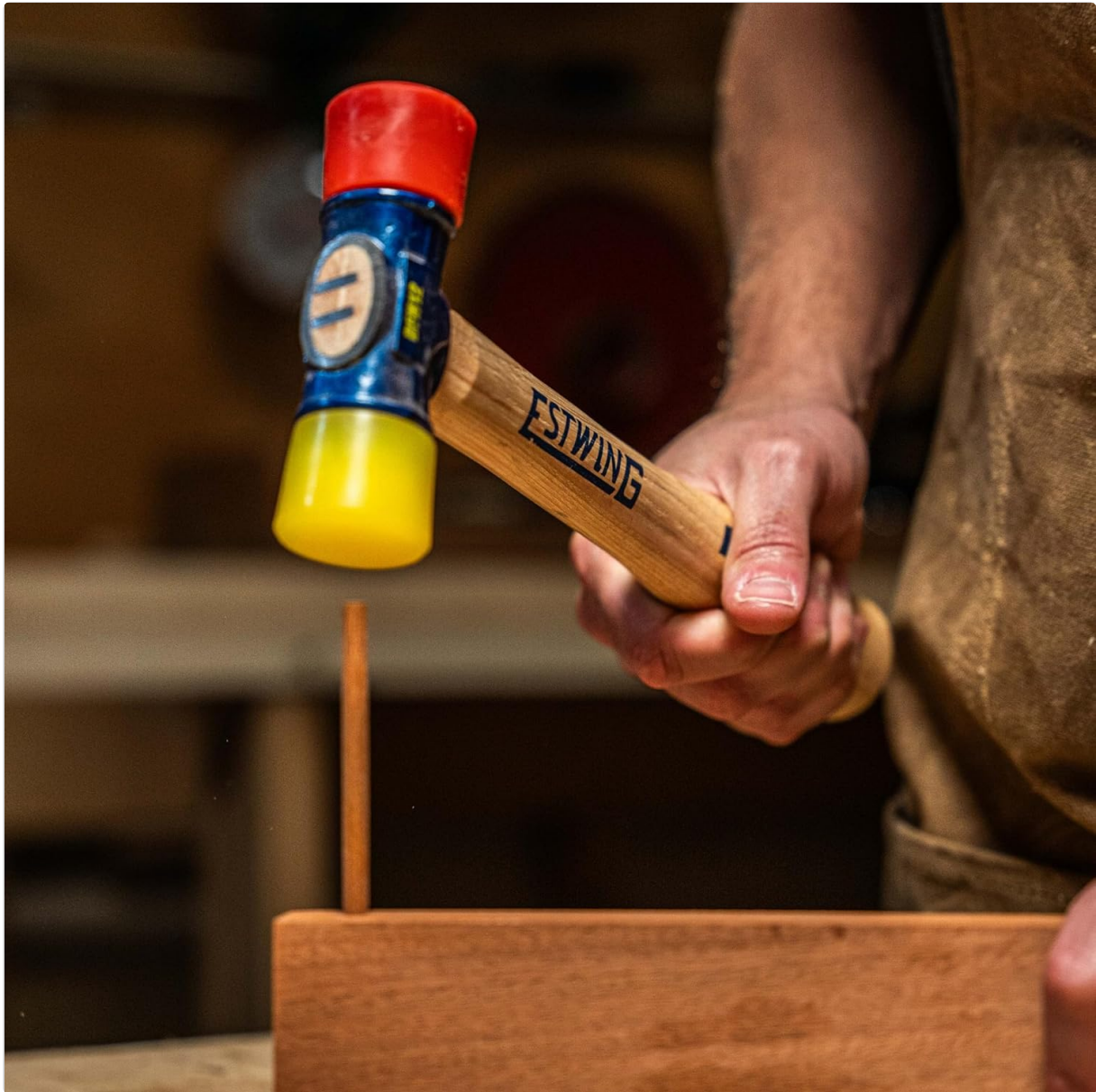
Figure 3: Using the mallet for dowel insertion
