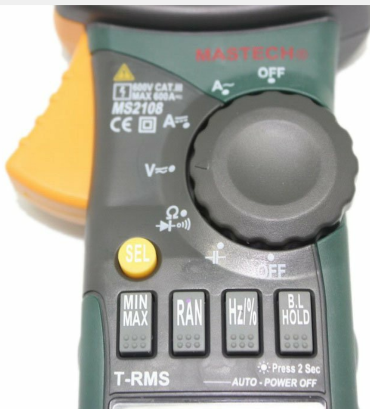
Close-up view of the control panel on the Mastech MS2108, detailing the function dial, SEL, MIN/MAX, RAN, Hz/%, and B.L. HOLD buttons.
