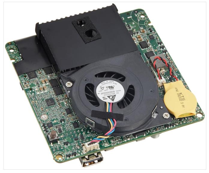
Figure 2: Rear view of the Intel D332 Desktop Motherboard, highlighting the integrated cooling fan and heatsink assembly.
