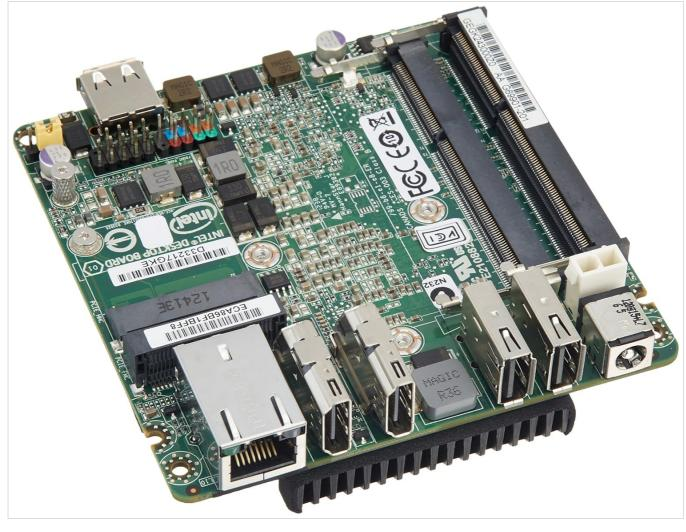
Figure 1: Front view of the Intel D332 Desktop Motherboard, showing the various ports, memory slots, and processor area.
