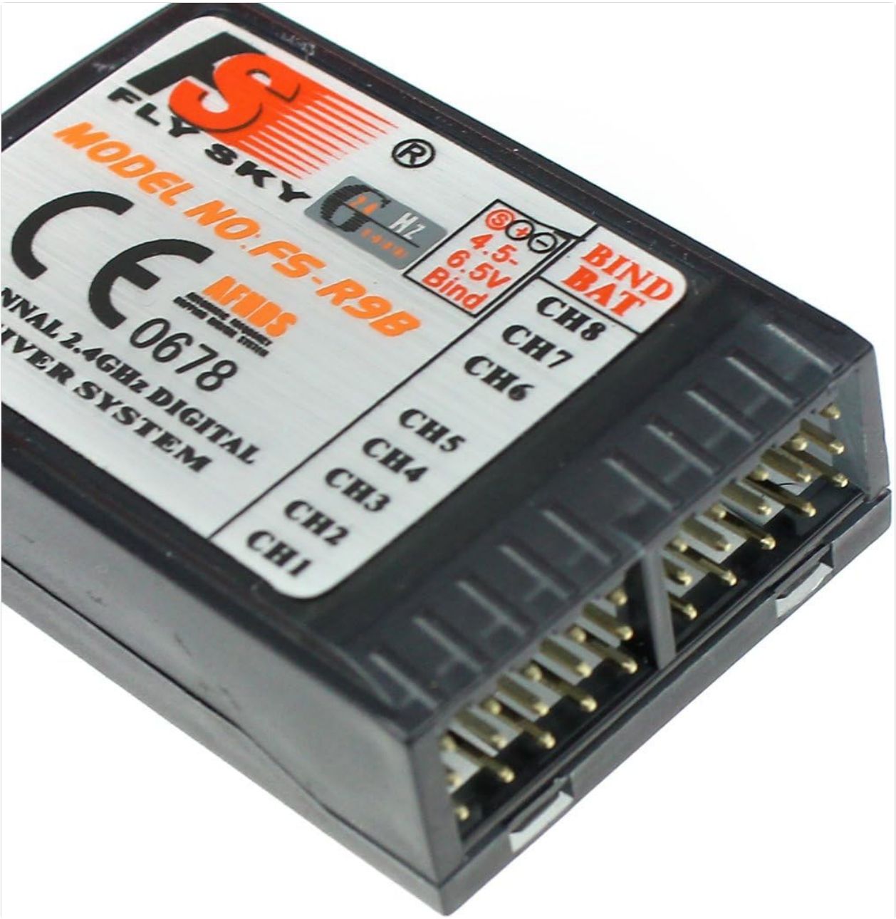
Image 4.1: Close-up view of the Flysky FS-R9B receiver's channel ports (CH1-CH8) and the BIND/BAT port.
