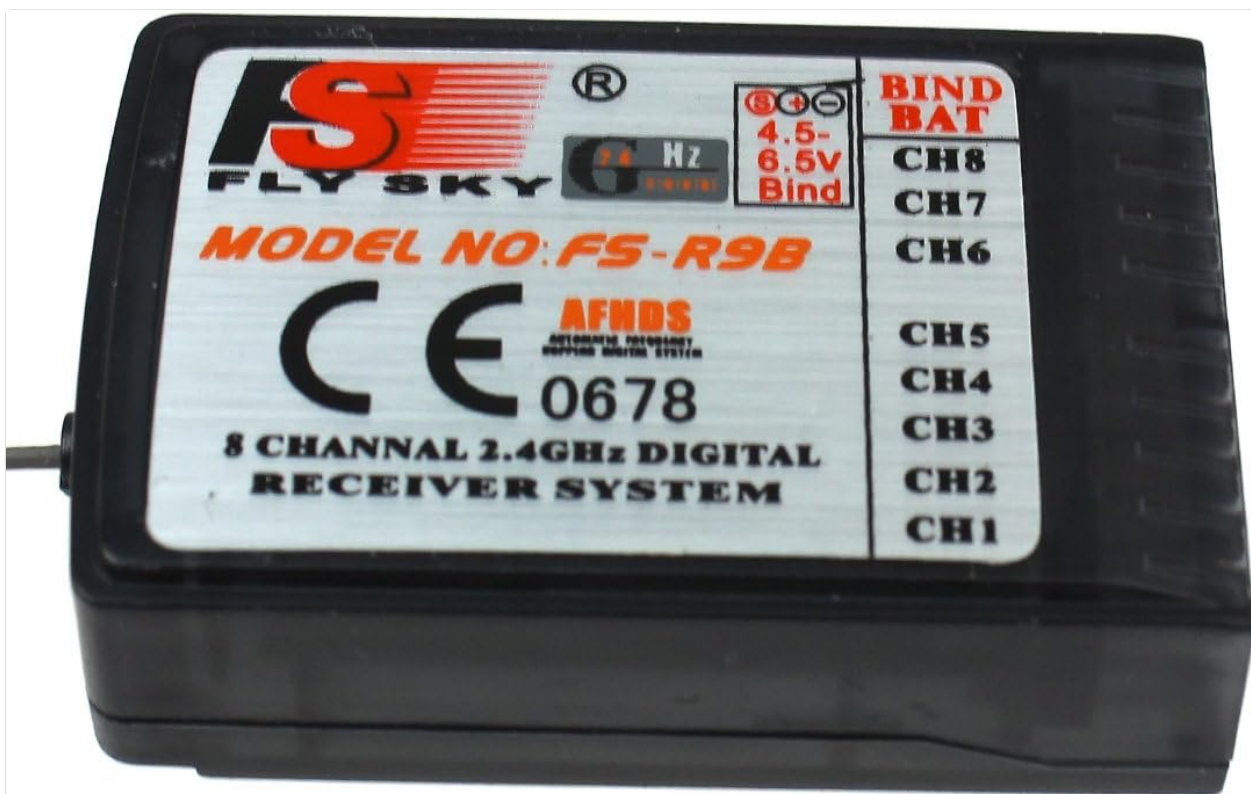
Image 1.1: Front view of the Flysky FS-R9B 8-channel receiver, showing the model number, CE certification, and channel labels.
