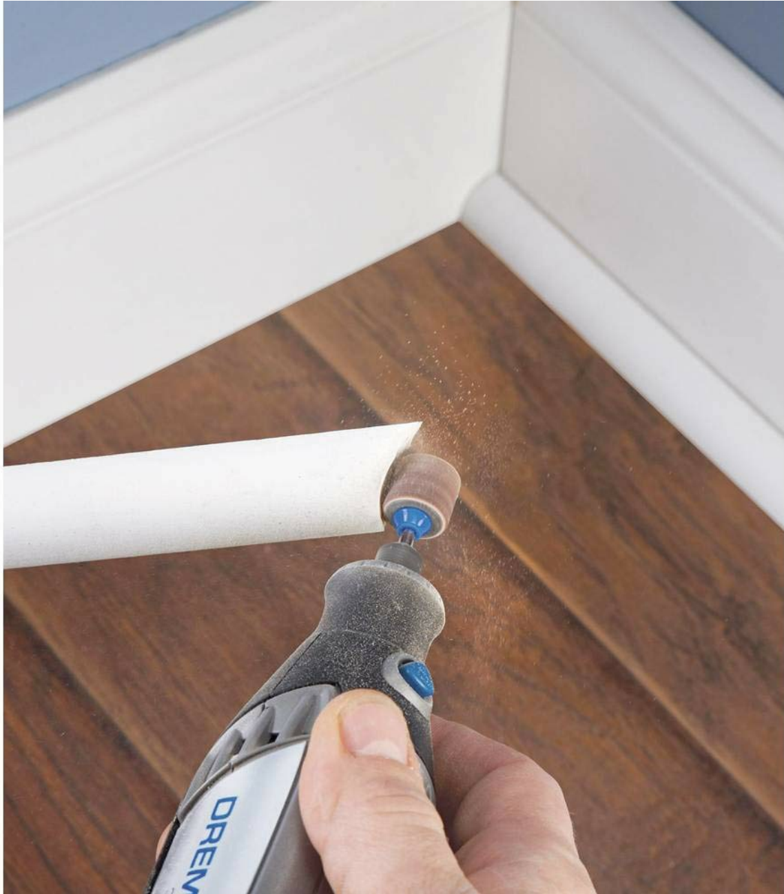
Figure 3: Dremel tool with EZ SpeedClic sanding band performing a sanding task.
