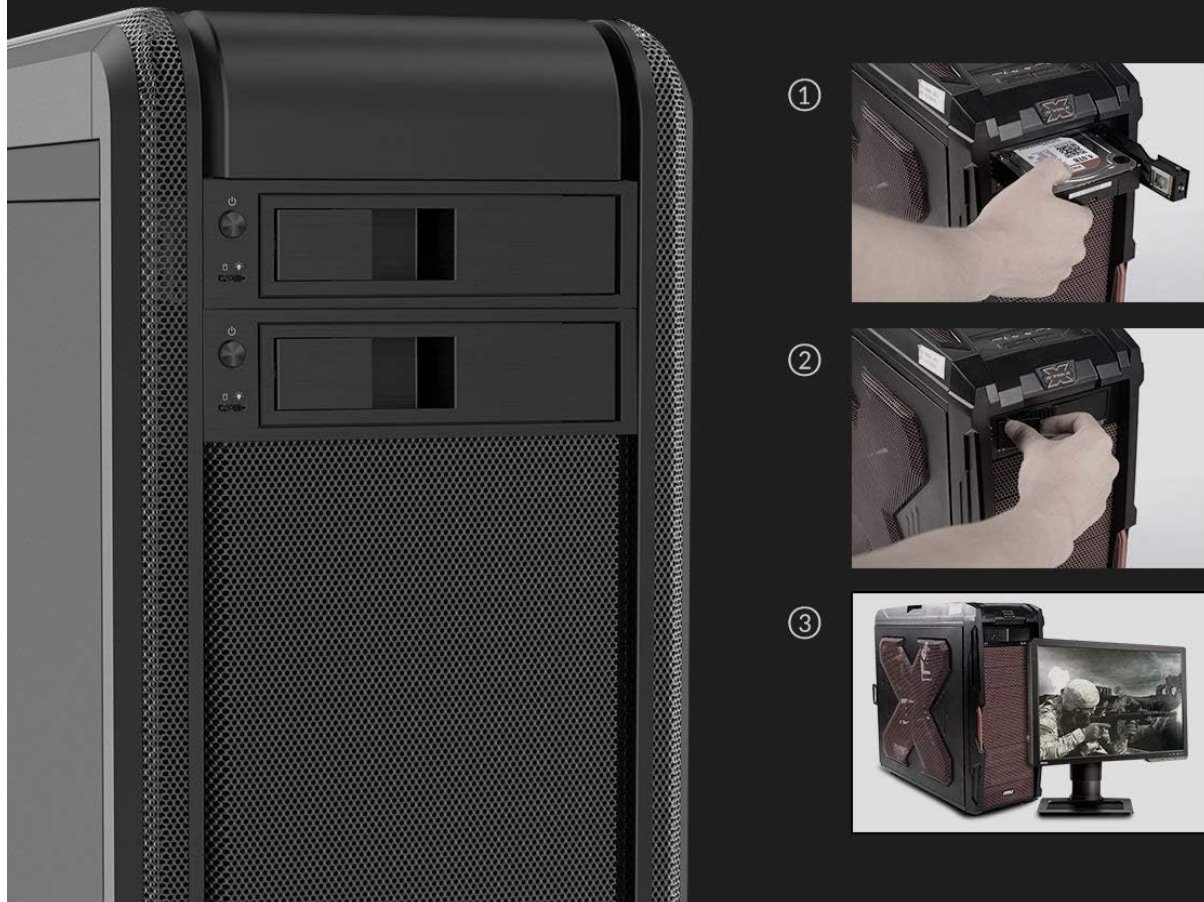
Image 2.1: Installation of the mobile rack into a computer's 5.25-inch drive bay.
