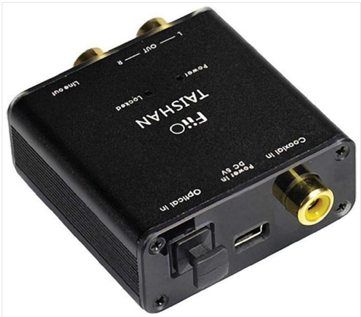
Image Description: A top-down view of the FiiO D3 (D03K) Digital to Analog Audio Converter. The device is black with gold-plated RCA output jacks (L and R) on one side, and coaxial and optical digital inputs on the other. A mini-USB power input is also visible. Status indicator lights for 'Power' and 'Locked' are present on the top surface.
