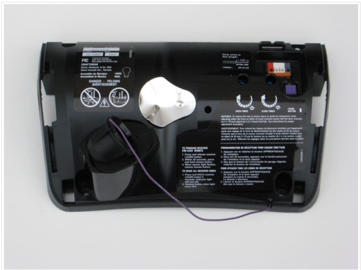
Image: The Sears Craftsman 41AB150-2 Receiver Logic Board, showing internal components, wiring, and printed safety warnings and programming instructions. The board is black with a metallic silver component and a purple wire.
