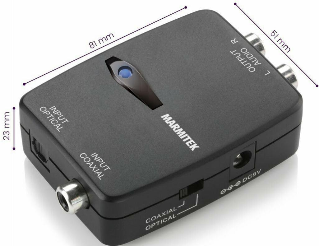
Figure 1: Overview of the Marmitek Connect DA21 with labeled ports and dimensions. The device measures 81mm in length, 51mm in width, and 23mm in height. It features an Optical Input, Coaxial Input, DC 5V power input, and L/R Audio Output (RCA).
