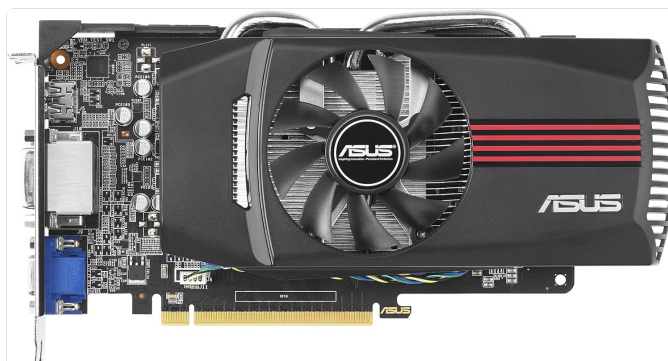
Figure 3.1: Top-down view of the ASUS GTX650-DC-1GD5 Graphics Card, showing the fan and PCB layout, useful for identifying connection points.
