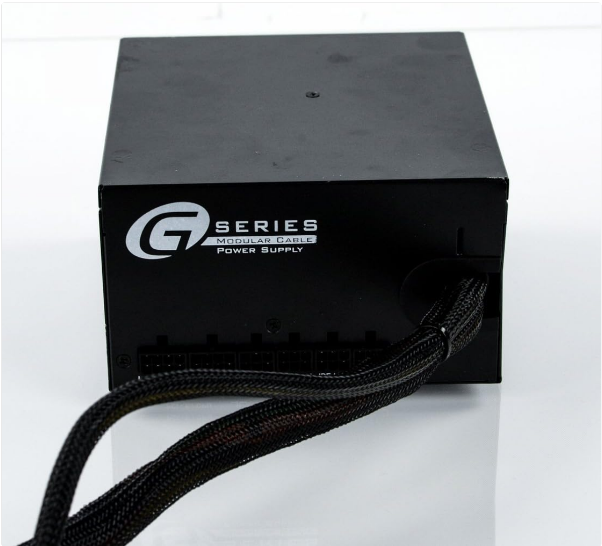
Image: The Seasonic G Series 550 power supply with a selection of its modular cables, ready for connection.
