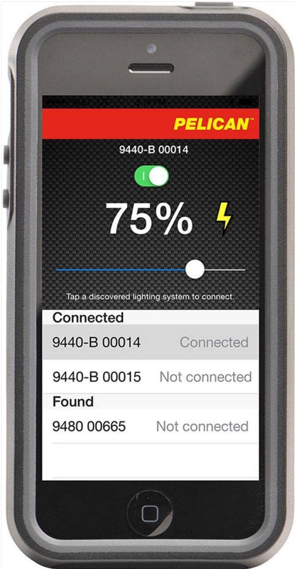
Figure 3.1: A smartphone interface showing the control application for the Pelican lighting system, including battery status and connection options.
