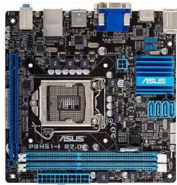
Figure 2: Angled view of the motherboard, showing the CPU socket, memory slots, and various headers.
