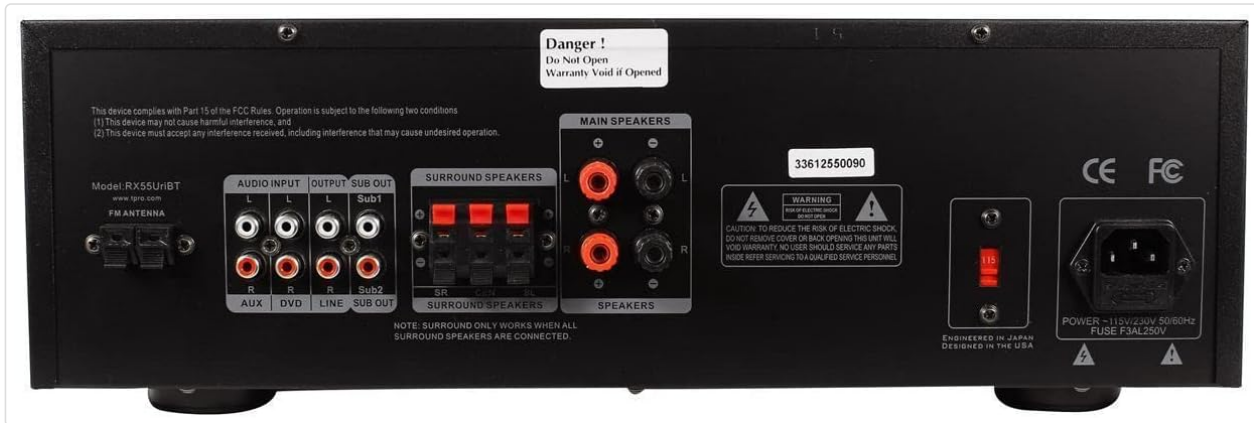
Figure 3: Rear Panel Connections. This image illustrates the rear connections, including RCA audio inputs (AUX, DVD, LINE), main speaker outputs (banana binding post), surround speaker outputs (push button), RCA line out, and mono RCA subwoofer outputs.
